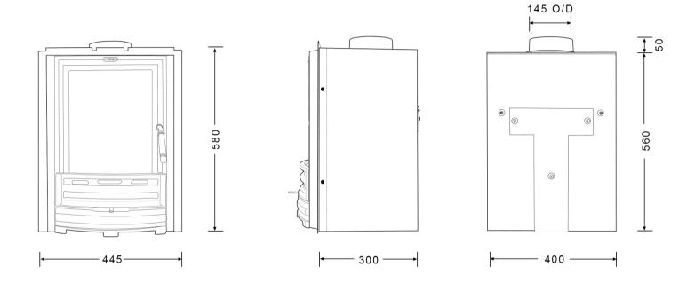
O/D = Outside Diameter Measurements in Millimetres
